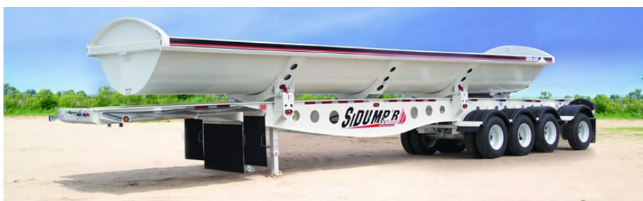
Quad-axle 48'10" length, 102" wide, 36' or 38' tub, 23-25 CU Yards capacity
